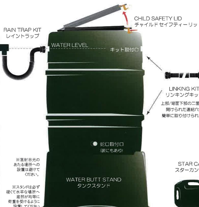
The Rain Trap is designed to fit into all regular downpipes of 60-100mm diameter plus 65mm square. The flexible connecting hose enables the water storage container to be redirected to a suitable drain or soakaway. The connector easily fits into the pre-drilled hole at the top of the Harcostar Water Storage container.
